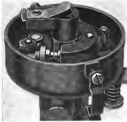
Left—The Connecticut complete assembly. Center—Removing the distributor head lays bare the breaker. Right—Diagrams of Connecticut breaker and of new advancing mechanism
